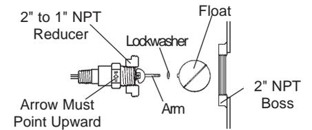
**Method B: When inside of tank is accessible.** Unscrew and remove float and lockwasher from unit arm. Insert unit in 1" NPT boss in tank and tighten so that arrow on housing points upward. Reassemble float and lockwasher on unit arm from inside of tank.
